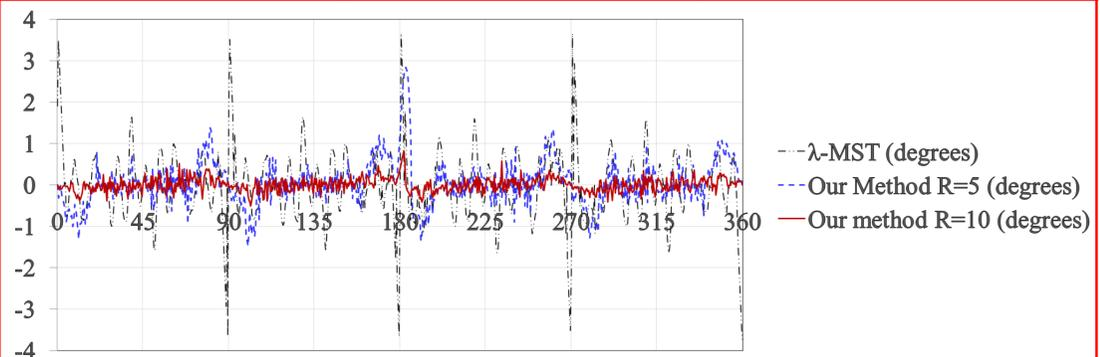
Average absolute error in the computation of tangents for 100 experiments with digitized circles of radius 100 and centers within 1 pixel region chosen randomly. The result is compared with  $\lambda$ -MST estimator.
